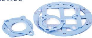
Durlon® 9007 is formulated with a homogenous blend consisting only of pre-shaped inorganic fillers, pure PTFE resins, and pigment. It is suitable for use in steel flanges and does not exhibit the cold flow problems associated with virgin PTFE of the hardness problems of silica-filled PTFE. Unlike generic glass fibre filled PTFE, the shapes of the fillers used in Durlon® 9007 do not allow wicking of media through the gasket which can lead to corrosion on flange surfaces.
